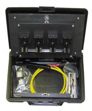
The probe, standards, and batteries are stored inside the ES Meter case. Twist the lock to open the door and access these items.
